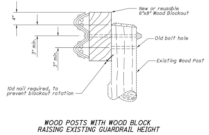
Alternate methods of placing the Blockouts on round Posts may be submitted for consideration and approved by the Engineer.
